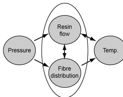
Figure 1: Relation between processing conditions and fibre/resin distribution
