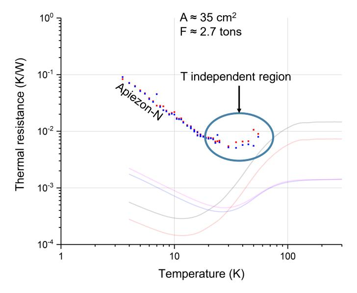
20 – 50 K range measured accurately after heater upgrade (3 W → 10 W)
