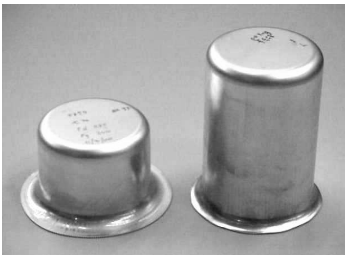
Figure 1: Limiting drawing results at 20 °C (left) and with the flange at 250 °C (right).
