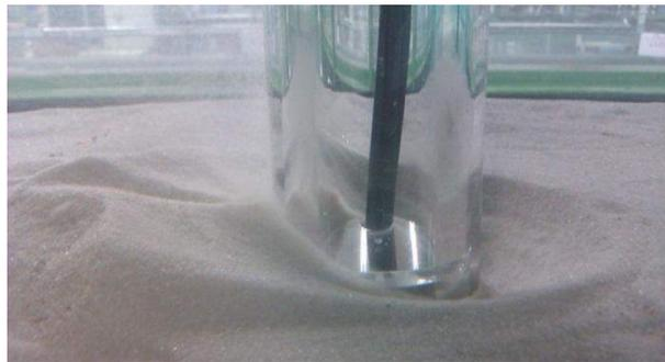
Figure 1. Initiation of scour hole formation during experiment
