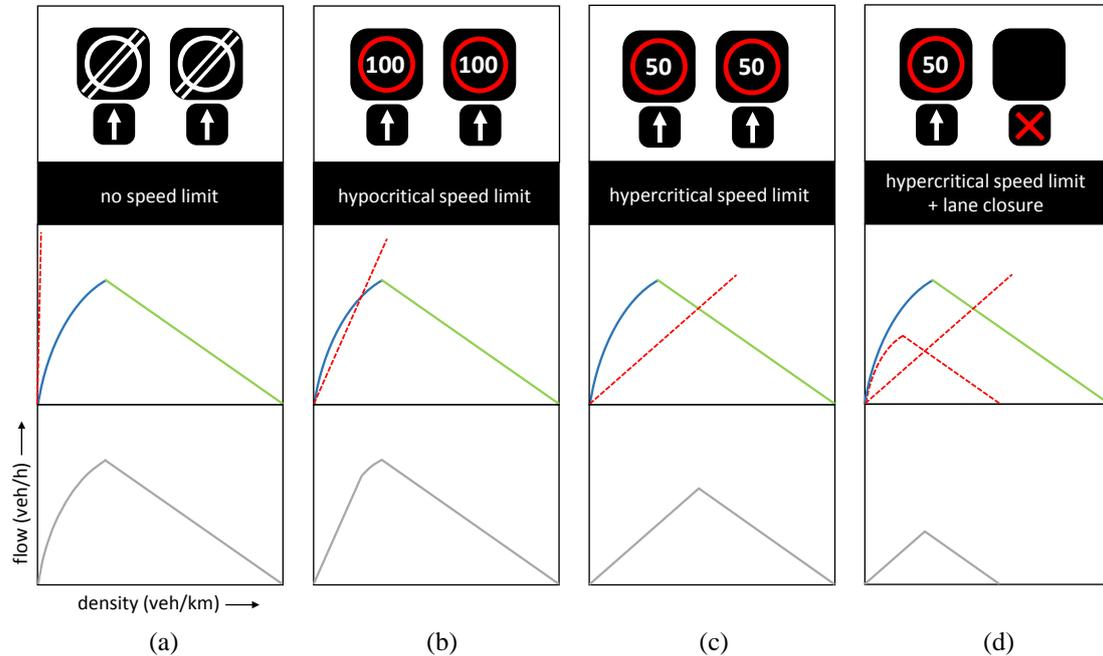
**Figure 1** Constrained fundamental diagrams in case of (a) no speed limit, (b) hypocritical speed limit, (c) hypercritical speed limit, (d) hypercritical speed limit and lane closure.
