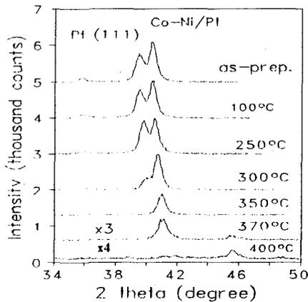
Fig.2 High-angle XRD patterns of a series of annealed samples. The layer thicknesses as sputtered are  $235 \text{ \AA Pt} + (6.3 \text{ \AA CoNi} + 14.7 \text{ \AA Pt}) \times 17$
