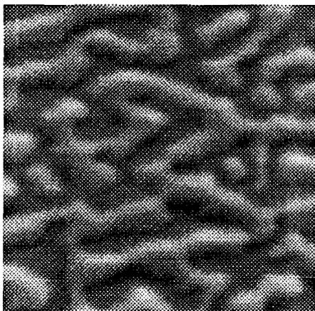
Fig 4. MFM image of a typical domain pattern in the unannealed, high coercivity sample (A:  $235 \text{ \AA Pt} + (3.8 \text{ \AA CoNi} + 5.9 \text{ \AA Pt}) \times 17$ ) after demagnetization. The size of the scanned area is  $3 \times 3 \text{ \mu m}$ . The rough domain walls indicate the influence of pinning effects during the remagnetization process.
