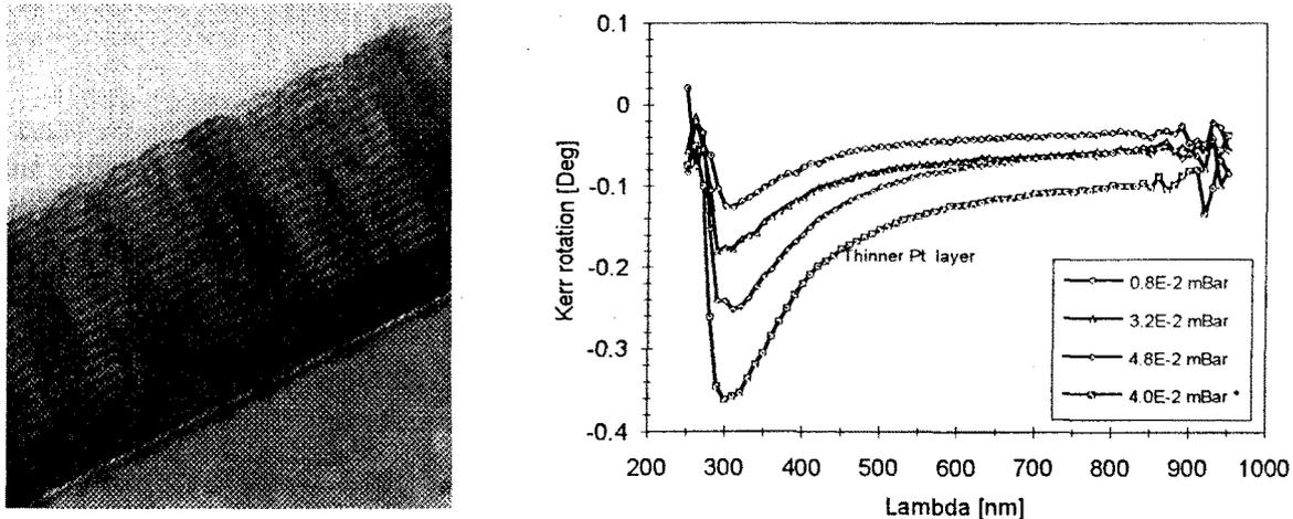
Fig.1. a) Cross section TEM micrograph of 17 CoNi (3.75 nm)/Pt(1.47nm) bilayers on a 23.5 nm Pt seedlayer on Si.
