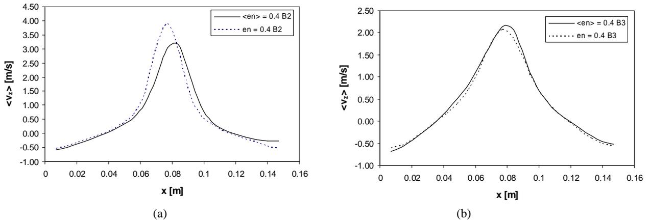
**Figure 8:** Time-averaged vertical particle velocity profile for different variable restitution coefficients compared to constant restitution coefficients for case B2, the spouting-with-aeration regime (a) and case B3, jet-in-fluidized-bed regime (b) at  $z = 0.15$ .
