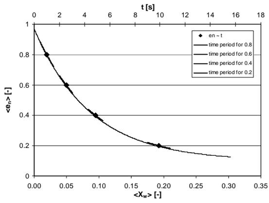
**Figure 2:** Overall restitution coefficient versus time and average moisture load. The chosen time-period per stage of the granulation or wetting process is visualized.
