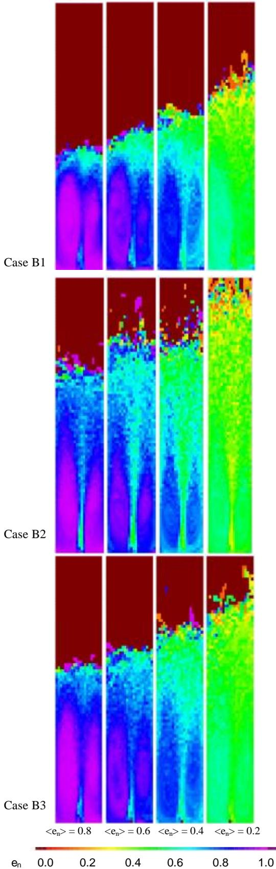
**Figure 4:** Time-averaged restitution coefficient per grid cell for different variable restitution coefficients for case B1 (intermediate / spout - fluidization regime), B2 (spouting-with-aeration regime) and B3 (jet-in-fluidized-bed regime) at different stages of the wetting process, distinguished by the overall restitution coefficient  $\langle e_n \rangle$ .
