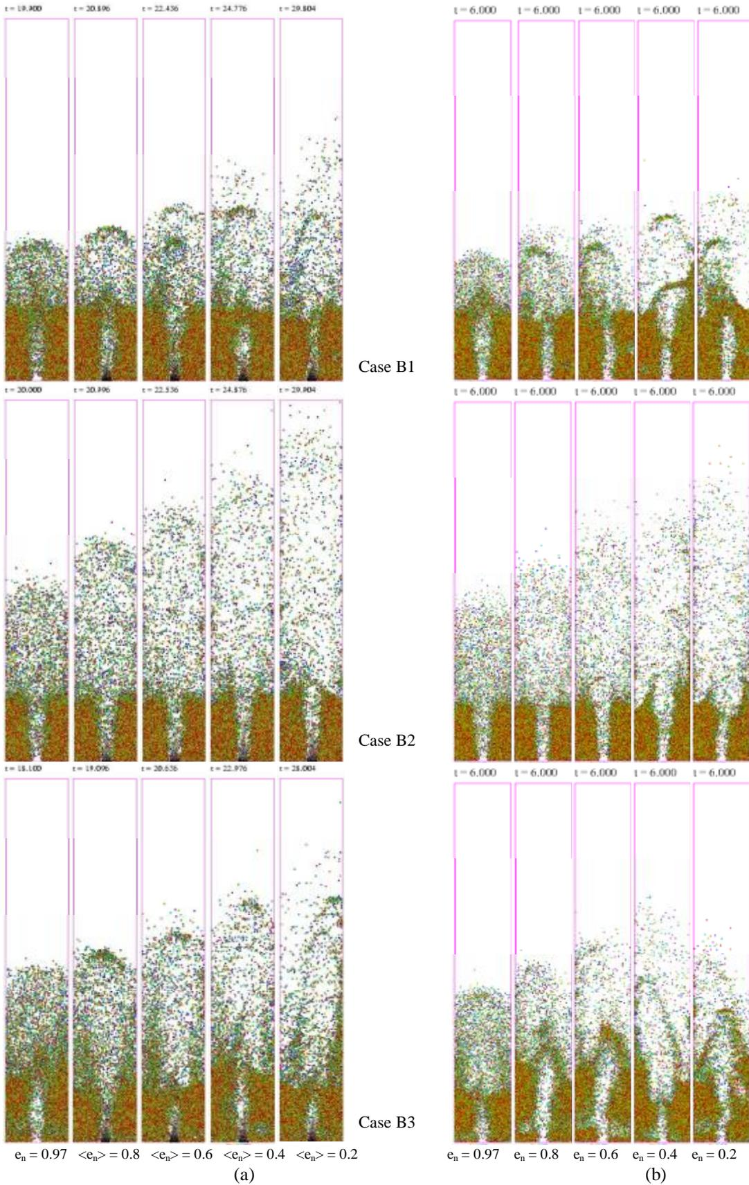
**Figure 3:** Snapshots of the simulated instantaneous particle positions for different variable restitutions (a) at different stages of the wetting process distinguished by the overall restitution coefficient  $\langle e_n \rangle$  and different constant restitutions (b) at simulation time  $t = 6$  s for case B1 (intermediate / spout - fluidization regime), B2 (spouting-with-aeration regime) and B3 (jet-in-fluidized-bed regime).
