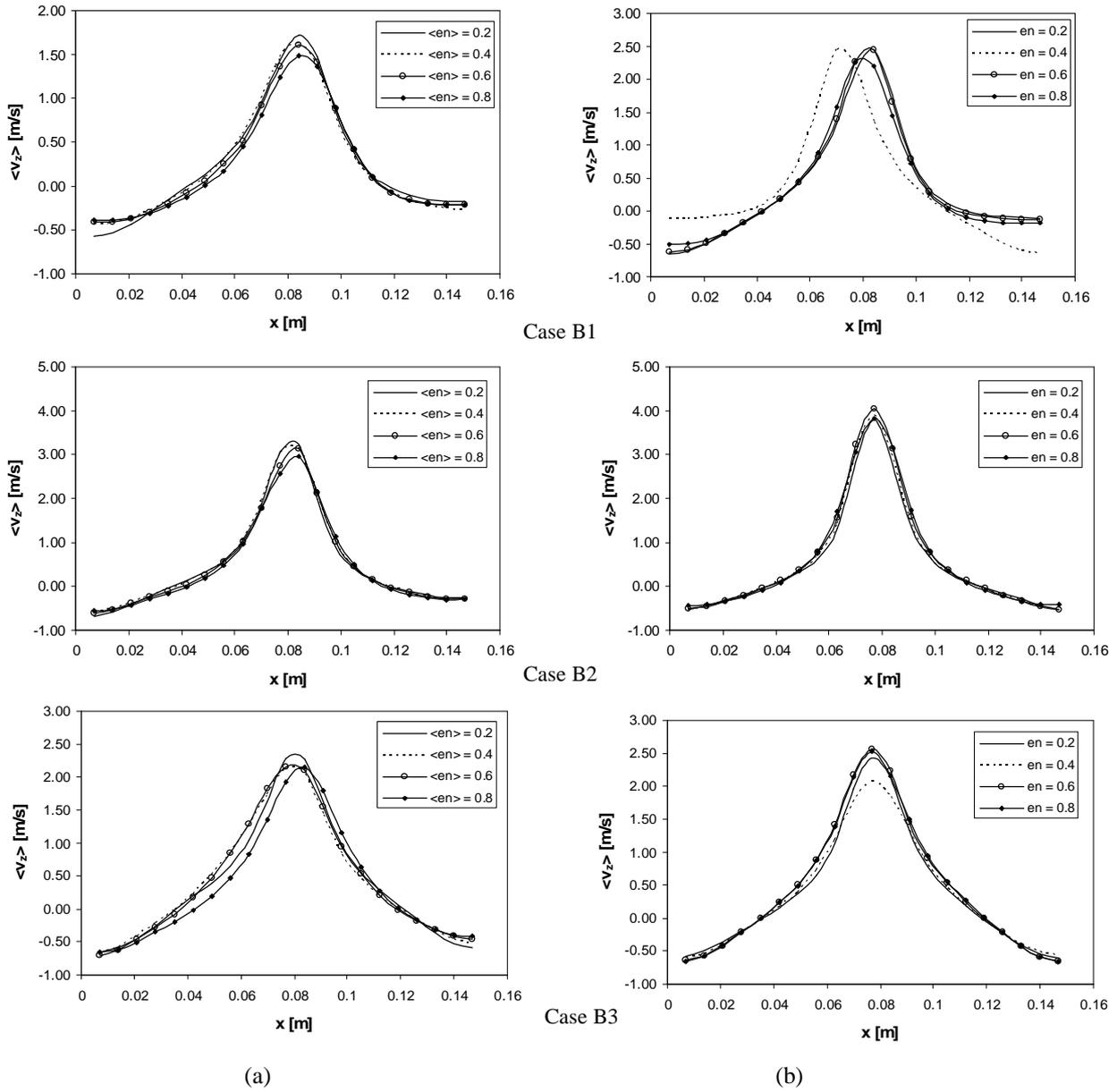
**Figure 7:** Profiles of the time-averaged vertical particle velocity for different variable (a) and constant (a) restitution coefficients at  $z = 0.15$  for case B1 (the intermediate /spout-fluidization regime), B2 (spouting-with-aeration regime) and B3 (jet-in-fluidized-bed regime).
