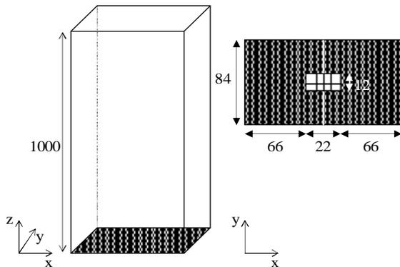
**Figure 1:** Schematic representation of the geometry of the 3D spout fluidized bed, dimensions are given in mm.
