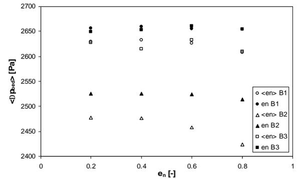
**Figure 6:** Time-averaged pressure drop for different constant restitution coefficients ( $e_n$  as reported in Van Buijtenen et al. (2007)) and different variable restitution coefficients at different stages of the wetting process, distinguished by the overall restitution coefficient  $\langle e_n \rangle$ , for case B1 (intermediate / spout - fluidization regime), B2 (spouting-with-aeration regime) and B3 (jet-in-fluidized-bed regime).
