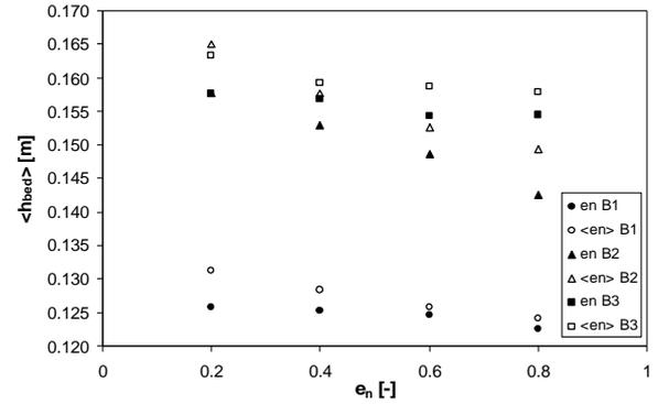
**Figure 5:** Time-averaged bed height for different constant restitution coefficients ( $e_n$  as reported in Van Buijtenen et al. (2007)) and different variable restitution coefficients at different stages of the wetting process, distinguished by the overall restitution coefficient  $\langle e_n \rangle$ , for case B1 (intermediate / spout - fluidization regime), B2 (spouting-with-aeration regime) and B3 (jet-in-fluidized-bed regime).
