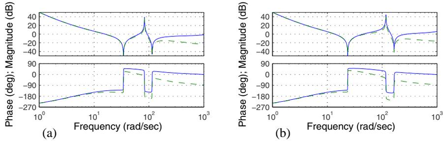
Figure 4: Bode plots of the open loop SISO system for actuator 1. The solid lines are with the PID controller of Eq. (14); the dashed lines are with an additional pole in  $-1/\alpha_i\tau_{D,i}$ . Graph (a) is for the initial configuration and (b) for the final configuration.
