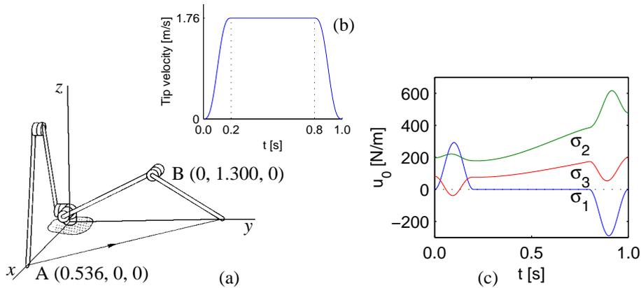
Figure 2: (a) Motion trajectory and (b) velocity profile of the manipulator tip. (c) Nominal torques  $\underline{u}_0$  for the three actuators.
