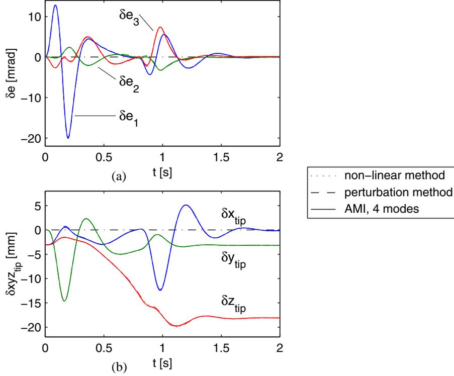
Figure 5: Deviation from the nominal trajectory according to three simulation methods: (a) actuator rotations and (b) tip co-ordinates.
