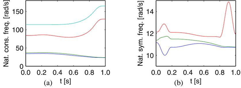
Figure 3: (a) Four lowest natural frequencies  $\omega_{c,i}$  for a constraint manipulator, Eq. (16). (b) Three lowest closed-loop natural frequencies  $\omega_i$  during the controlled trajectory motion of the manipulator computed with a symmetric  $\bar{K}_0^S$  as in Eq. (11).
