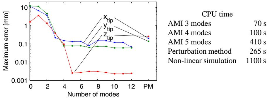
Figure 6: Maximum errors in the co-ordinates of the tip position as functions of the number of modes. The error is computed by comparing the AMI method with the perturbation method. For comparison the dots indicated with “PM” show the maximum difference between the perturbation method and the non-linear simulation. The table on the right illustrates the amount of CPU time for some of the simulations.
