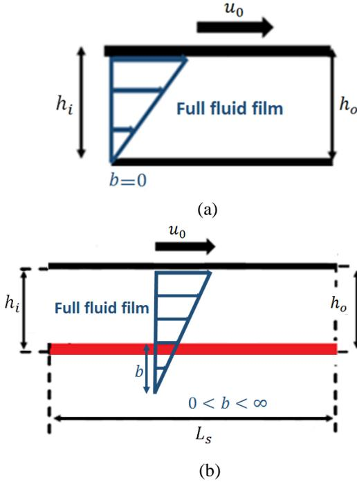
Figure 1: Schematic of wall slip model. (a) No-slip, (b) Boundary slip condition.
