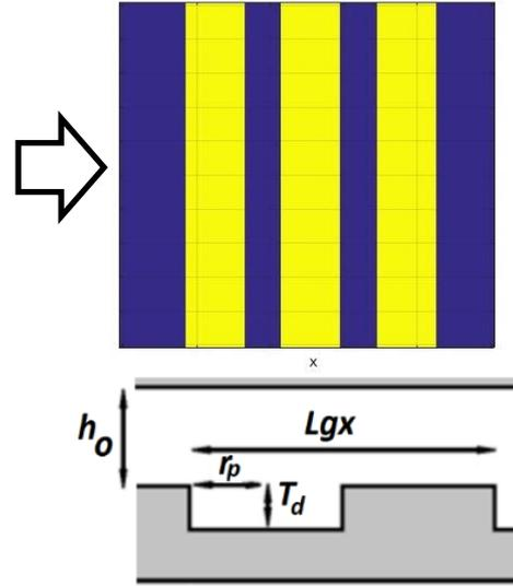
Figure 3: Texture pattern (open groove pattern).
