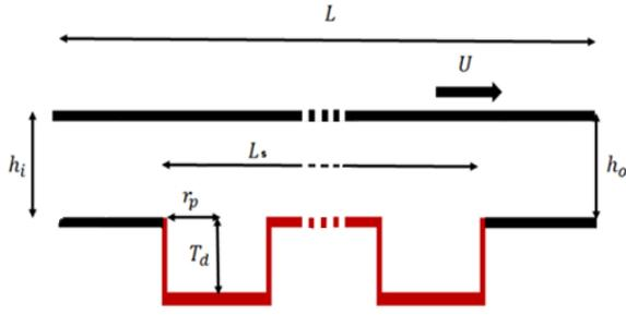
Figure 2: The schematic parallel sliding contacts, the red lines are showing the surfaces with boundary slip effect.
