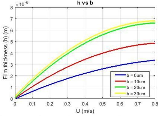
Figure 4: Influence of slip length on film thickness.
