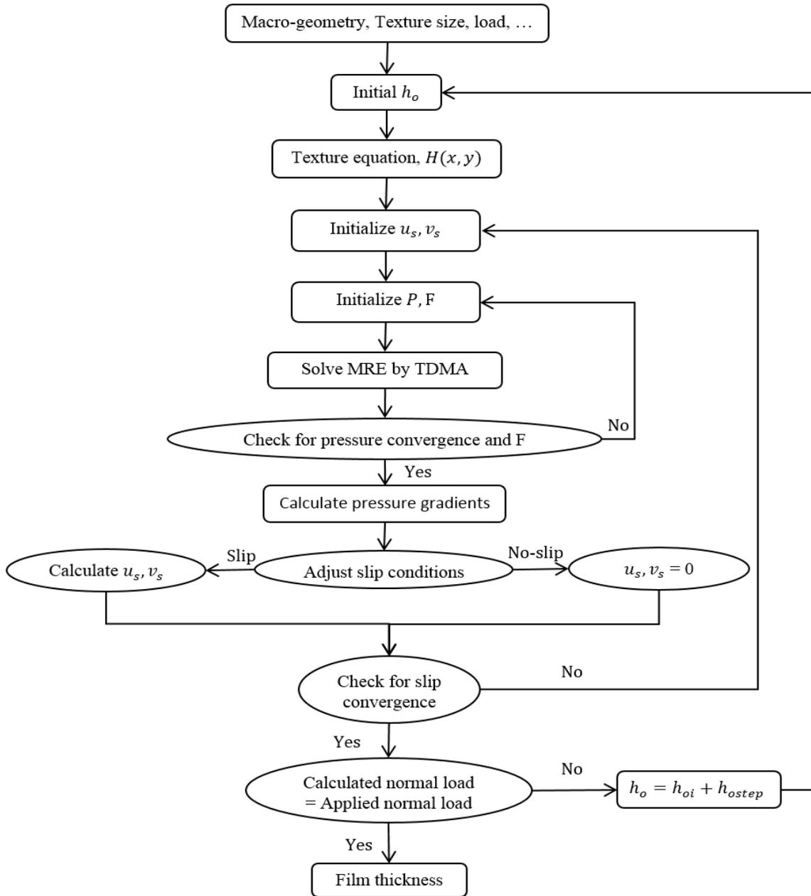
Figure A.1: Solution scheme for numerical calculations.
