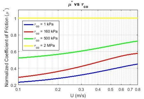
Figure 7: Influence of critical shear stress on friction.
