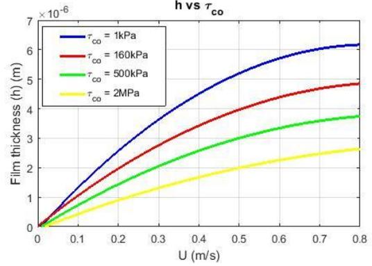
Figure 6: Influence of critical shear stress on film thickness.
