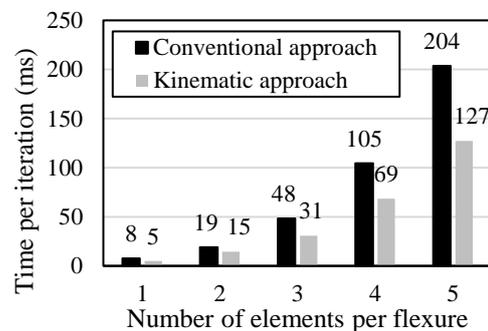
Figure 3. The average time per load iteration to obtain the deformed configuration.
