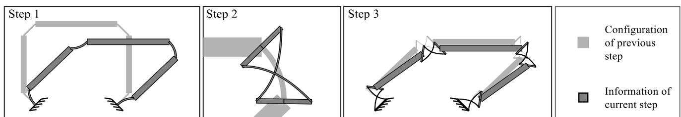
Figure 1. Schematic overview of the three steps in the method for the fourbar mechanism.
