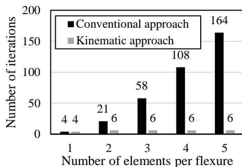
Figure 2. The minimal required number of load iterations to obtain the deformed configuration.
