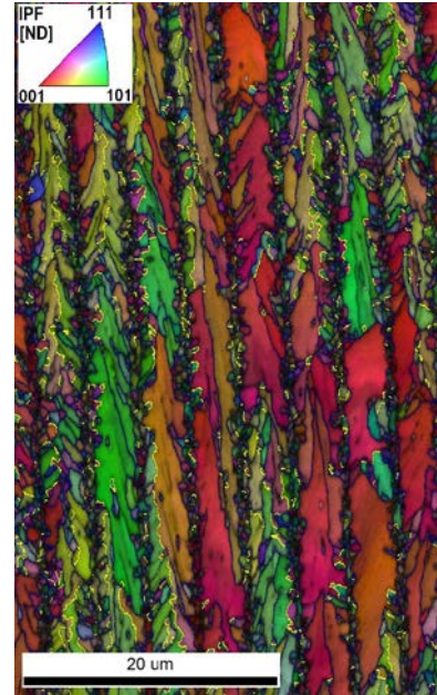
Fig. 4: Exemplary grain orientation map of a laser-crystallized 100-nm \text{Ge}_{0.85}\text{Si}_{0.15} film on \text{SiO}_2 , characterized by electron backscatter diffraction during top-view SEM imaging. (Colors indicate grain orientation as indicated in the legend). The laser beam scanned this sample in the vertical direction, leading to the formation of elongated crystal grains.
