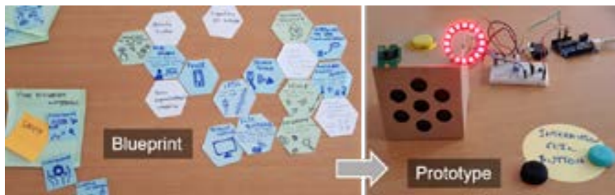
Figure 7. Liz designed a security, maintenance and well-being collaborative robot (system) that provides non-intrusive, task-oriented feedback through an LED ring or through localized button-activated speech
