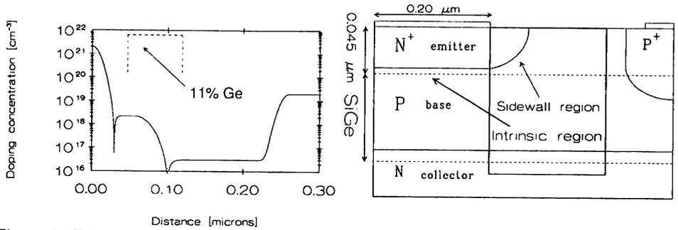
Figure 1: The vertical doping profile and cross-section of the NPN HBT/BJT. The full drawn lines are the emitter and collector junctions. The rectangular area drawn in the figure corresponds to the area used in the simulations shown in figure 2. The SiGe region is indicated with dotted lines. The distance in the vertical doping profile is relative to the poly-Si/mono-Si interface.
