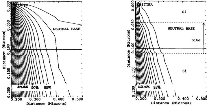
Figure 2: Current spreading at the emitter sidewall in the BJT (left figure) and the HBT (right figure) ( $W_e = 0.40\mu\text{m}$ ,  $V_{be} = 0.50\text{V}$ ,  $T = 300\text{K}$ ). The area of these figures corresponds with the rectangular area drawn in figure 1. The area between two current flow lines represents 1 % of the total current. The number under the flowlines gives the percentage of the total current that flows between the lines and the axis of symmetry.
