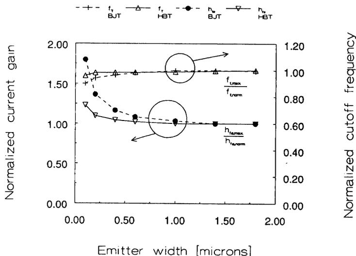
Figure 3: The normalized maximum cutoff frequency  $f_{t,max}/f_{t,norm}$  and maximum current gain  $h_{fe,max}/h_{fe,norm}$  as a function of the emitter width  $W_e$  for both the HBT and BJT simulated with MEDICI ( $V_{cb} = 1.0$  V and  $T = 300$  K). The normalization factors used for the HBT are  $h_{fe,norm} = 360$  and  $f_{t,norm} = 51$  GHz and for the BJT  $h_{fe,norm} = 60$  and  $f_{t,norm} = 39$  GHz.
