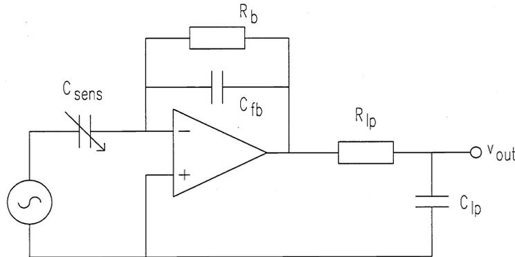
Figure 3.3.3 AM detection circuit for the accelerometer.
