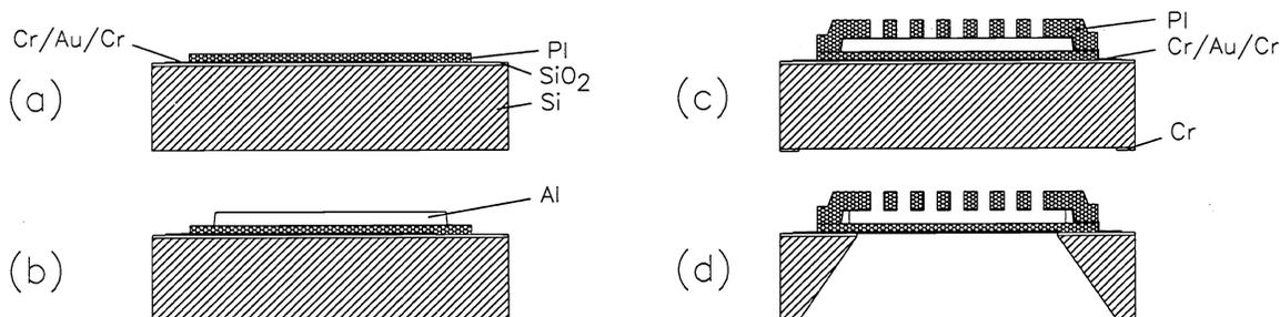
**Figure 3.1:** Polyimide sensor process. (a) Deposition of the first Cr/Au/Cr metal electrode and polyimide layer. (b) Deposition of Al sacrificial layer. (c) Deposition of the second Cr/Au/Cr metal electrode and polyimide layer, and deposition of Cr etch mask on the backside of the Si substrate. (d) Etching of Al sacrificial layer and Si substrate.
