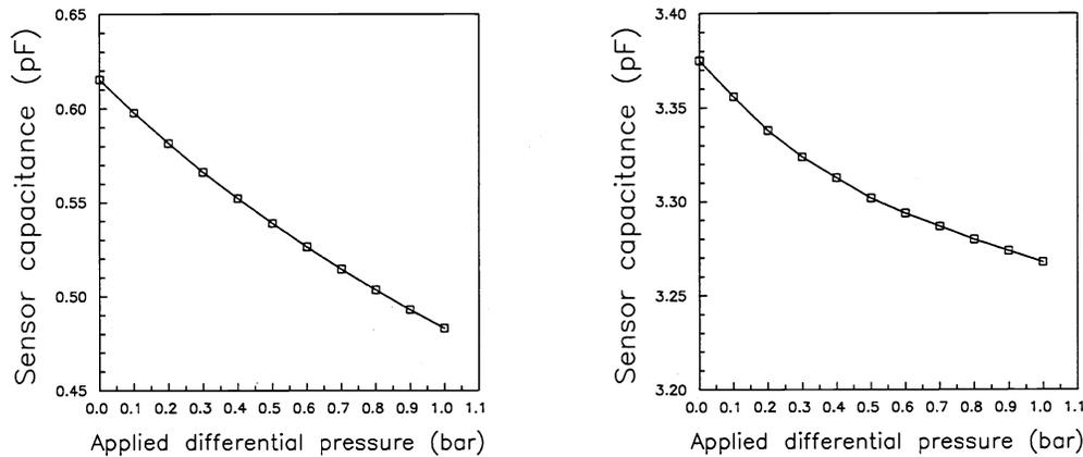
Figure 3.2.2: Calculated (left) and measured (right) capacitance of the pressure sensor vs. applied differential pressure.
