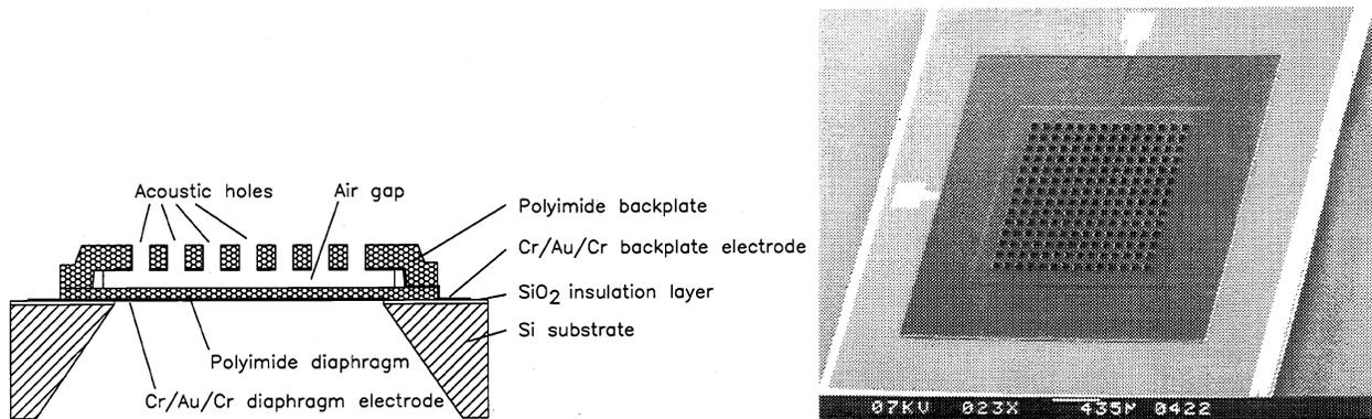
Figure 3.1.1: Cross-sectional view and SEM front view of the polyimide condenser microphone.
