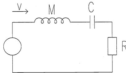
Figure 3.3.2: Mechanical equivalent circuit of the accelerometer.
