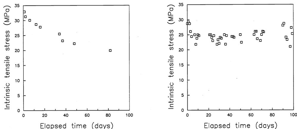
**Figure 2.2.1:** The average stress of HTR3 polyimide film vs. elapsed time. Left: Film cured in convection oven. Right: Film cured in 2 mbar N<sub>2</sub>.
