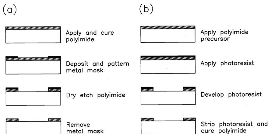
**Figure 2.1.1:** Processing of polyimide. (a) Patterning by dry etching. (b) Patterning by photolithography.
