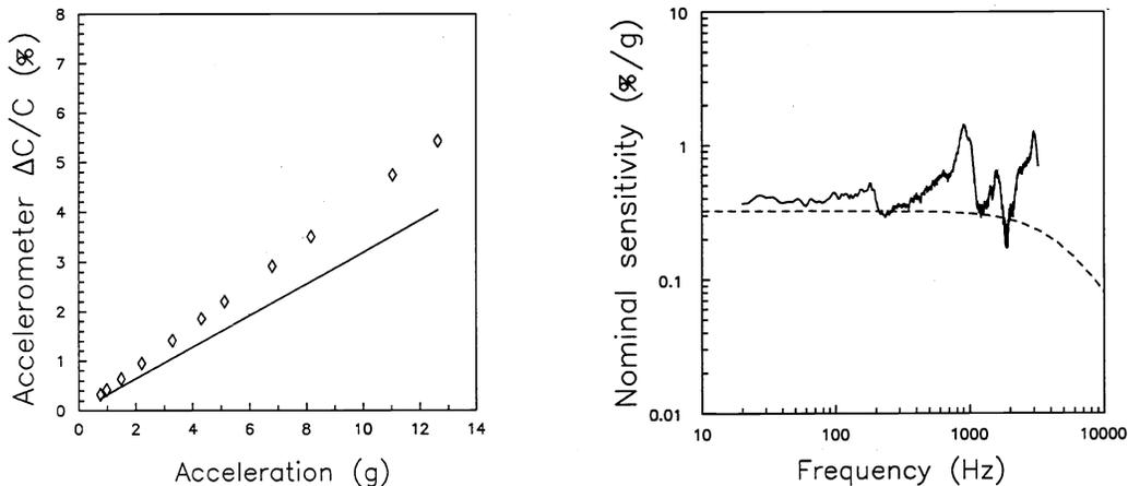
Figure 3.3.4: Change of capacitance vs. applied acceleration (Line: Theory.  $\diamond$ : Measurement), and frequency response (Dashed line: Theory. Solid line: Measurement) of the accelerometer.
