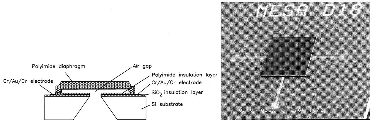
Figure 3.2.1: Cross-sectional view and SEM front view of the polyimide pressure sensor.
