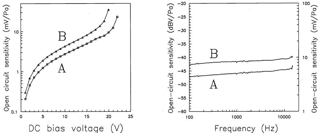
Figure 3.1.2: Measured characteristics of the polyimide condenser microphones. Left: Open-circuit sensitivity vs. DC bias voltage (frequency: 1 kHz). Right: Frequency response (DC bias voltage: 15 V). (A: 1.6 mm, B: 2.1 mm).
