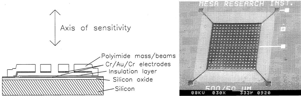
Figure 3.3.1: Cross-sectional view and SEM front view of the polyimide accelerometer.
