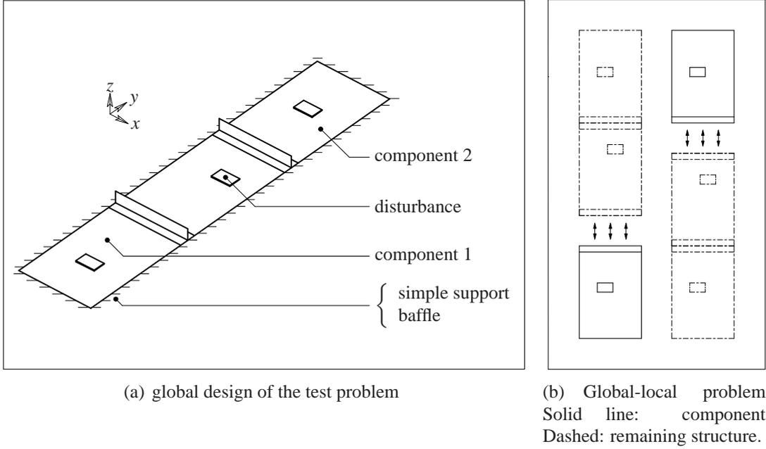
Fig. 3 The test problem: global design and global-local structure.
