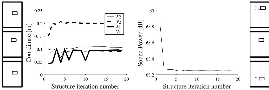
**Fig. 8** Results of broadband optimization. From left to right: Initial configuration, design variables, radiated sound power and result (solid line) superimposed on reference (dash-dot).
