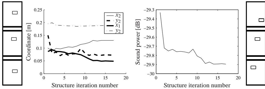
**Fig. 9** Results of harmonic optimization. From left to right: Initial configuration, design variables, radiated sound power and result.
