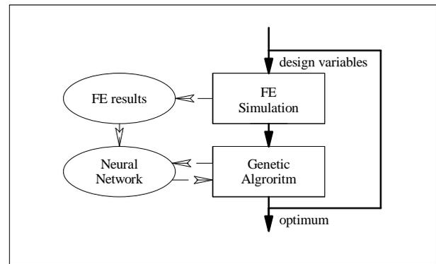
**Fig. 2** Component optimization (without selection method)
