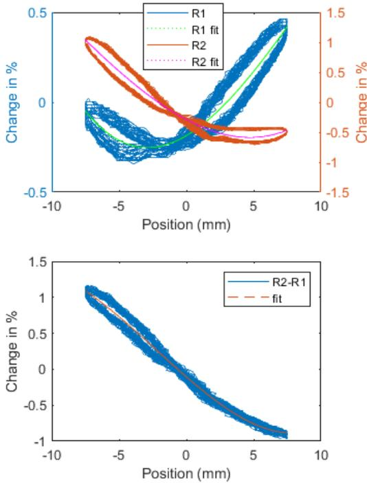
Fig. 5. Strongly reduced hysteresis due to differential measurement
