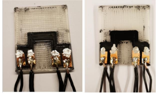
Fig. 2. Front and back side of the 3DP tactile sensor.
