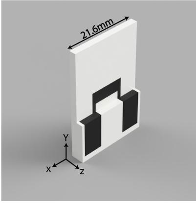
Fig. 1. 3D-model of the tactile sensor
