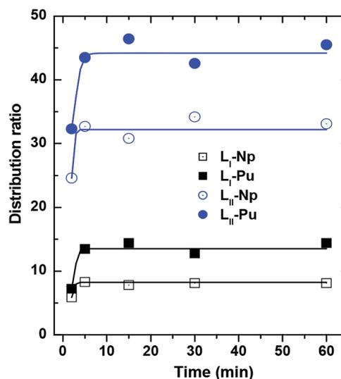
**Fig. 2** Distribution ratio of actinides by DGA ligands L<sub>I</sub> and L<sub>II</sub> showing the extraction kinetics for reaching the equilibrium condition. Organic phase: 1.0 mmol L<sup>-1</sup> ligands in 95% *n*-dodecane + 5% isodecanol; aqueous phase: 1 M HNO<sub>3</sub>.
