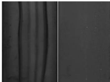
**Fig. 1.** Mixing of two flows: without (left) and with mixer (right)
