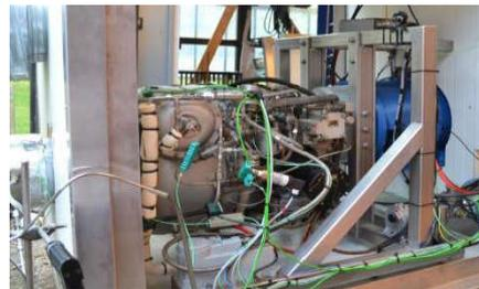
**Fig. 2.** Gas turbine test-rig
