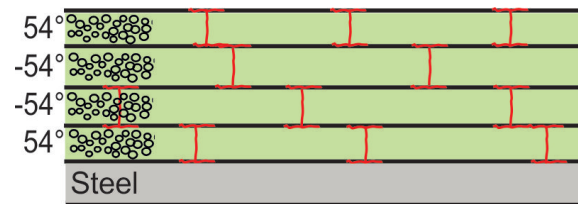
Figure 1. Crack formation and delamination in a FML. The black circles schematically indicates the glass fibres, the red lines cracks in the polymer matrix and delamination fronts in between the plies.
