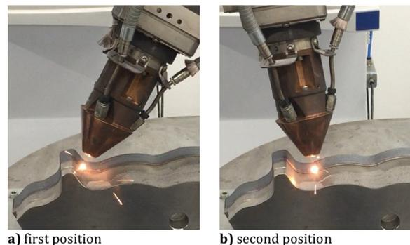
Fig. 3. Significant orientation change during a move.
