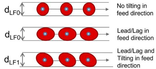
Fig. 2. Laser spot shape and dimensions depending on whether lead/lag and tilt are applied.
