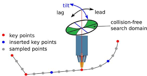
Fig. 1. Initialization of key point and initial orientation.
