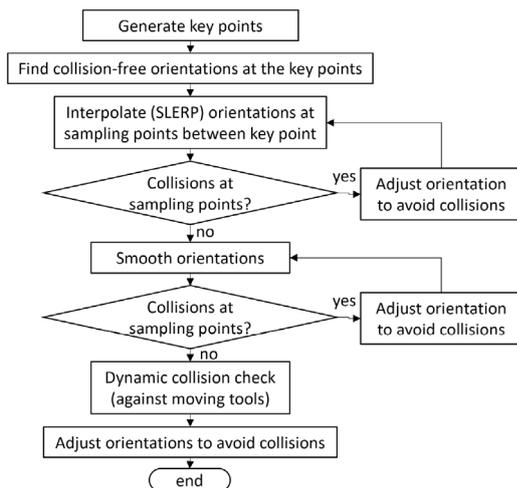
Fig. 5. Workflow of the algorithm.
