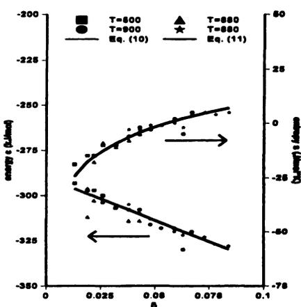
Fig. 7 Energy and entropy of oxygen incorporation in  $\text{La}_{0.8}\text{Sr}_{0.2}\text{CoO}_3$  as a function of oxygen nonstoichiometry
