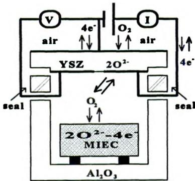
Fig. 1 Schematic plot of cell-1 used for coulometric titration experiments
