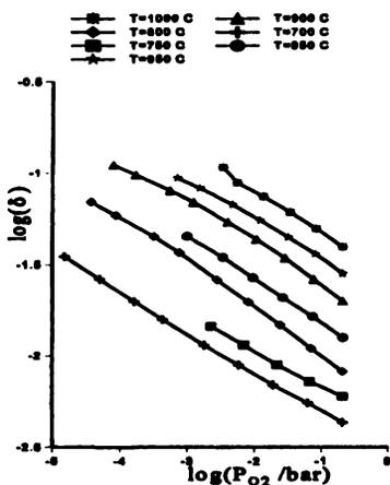
Fig. 6 Oxygen nonstoichiometry of  $\text{La}_{0.8}\text{Sr}_{0.2}\text{CoO}_3$  as a function of oxygen partial pressure and temperature
