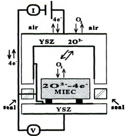
Fig. 2 Schematic plot of cell-2 used for coulometric titration experiments
