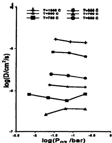
Fig. 4 Chemical diffusion in  $\text{La}_{0.8}\text{Sr}_{0.2}\text{CoO}_3$  as a function of oxygen partial pressure and temperature
