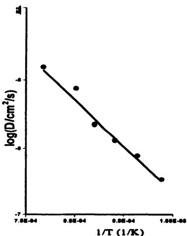
Fig. 5 Average chemical diffusion in  $\text{La}_{0.8}\text{Sr}_{0.2}\text{CoO}_3$  as a function of temperature
