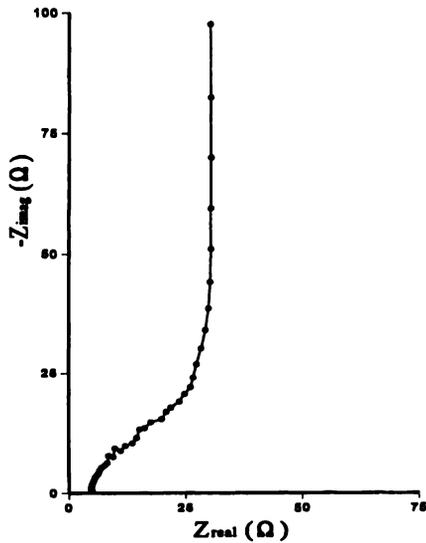
Fig. 3 Typical impedance plot including gas-phase capacitance, resistance and finite length diffusion impedance element
