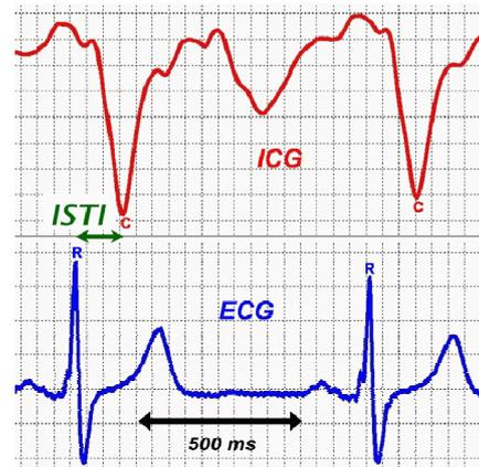
**Figure 2.** A typical example of simultaneous registration of an Impedance CardioGram (ICG) and an ElectroCardioGram (ECG) (arbitrary units). The marker points R in the ECG and C in the ICG are indicated. From these points the Initial Systolic Time Interval (ISTI) is determined, which can be considered as a measure of the time lag between the electrical and mechanical activity of the heart.
