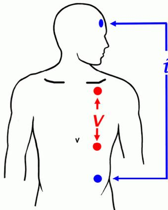
**Figure 1.** Electrode configuration: A small AC current (0.3 mA, 64 kHz) is applied to the thorax by means of the two outer electrodes. The two inner electrodes measure the subsequent electrical voltage difference over the heart. The impedance recording is obtained from the time course of this voltage signal. The ECG-signal is obtained from the two inner electrodes.
