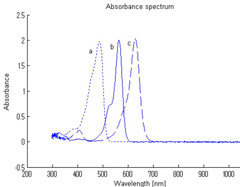
Fig.2. Absorption spectra of 13.0 mg/l of Disodium Fluorescein (DF), 15.0 mg/l Kiton Red (KR) and 13.0 mg/l Simacid Blue (SB).
