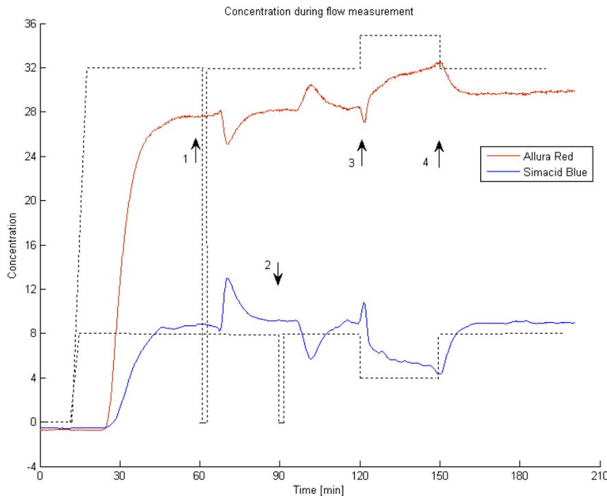
Fig.3. Absorption spectra of 40.0 mg/l Allura Red (AR) and 40.0 mg/l Simacid Blue (SB) in infusion measurement. Dotted line indicates the concentration input values.
