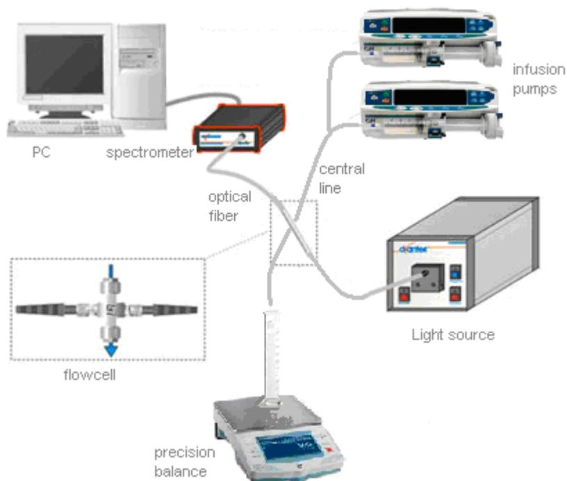
Fig.1. schematic view of experimental setup
