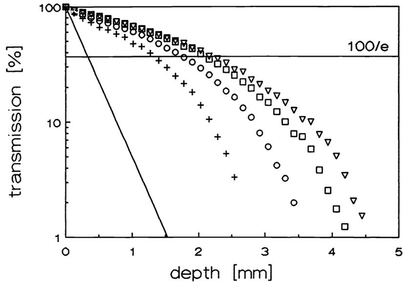
Figure 3: Transmission (in percent) of Holmium laser pulses delivered from a 320  $\mu\text{m}$  fiber tip submerged in saline as function of the thickness of the saline layer between fiber tip and bottom of the glass tray (depth in mm) for various intensities. +, 250 mJ/pulse, o, 500 mJ/pulse; □, 750 mJ/pulse and ▽, 1000 mJ/pulse. The solid line represents the theoretical transmission for low intensity Holmium laser pulses.
