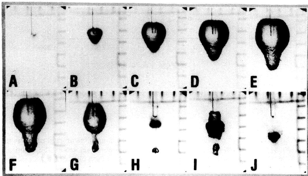
Figure 4: Vapour cavity expansion and implosion during a 0.75 J laser pulse (500  $\mu\text{s}$  total pulse duration, 200  $\mu\text{s}$  FWHM) delivered from a 320  $\mu\text{m}$  fiber submerged in saline. Photo A was taken at 15  $\mu\text{s}$ , B at 50, C at 100, D at 150, E at 250, F at 300, G at 400, H at 450, I at 600 and J at 850  $\mu\text{s}$  after the start of the laser pulse. Note the millimeter scales next to the fiber tip.
