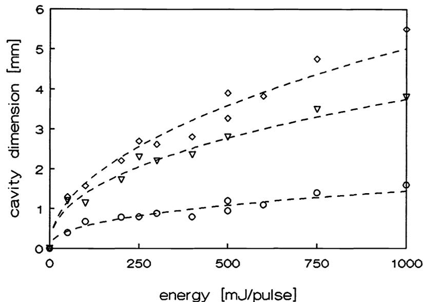
Figure 5: The maximum length (◇), depth (▽) and horizontal radius (○) of the vapor cavity as a function of the energy per pulse delivered from a  $320\ \mu\text{m}$  fiber tip.
