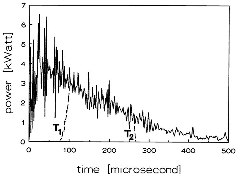
Figure 1: The temporal shape of a 1.00 J Holmium-YSGG laser pulse. The dotted line represents the estimated temporal shape of a laser pulse transmitted through 1.0 mm of saline.  $T_1$  is the time of onset of complete power transmission through the water vapor cavity and  $T_2$  is the timing of collapse of the vapor cavity.
