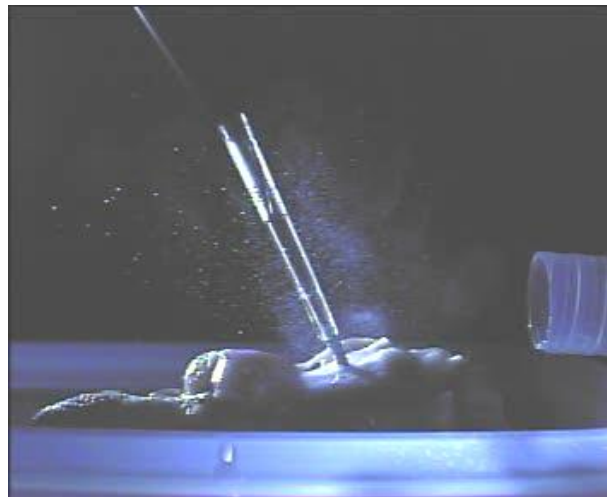
Figure 9. Using the special lighting technique, a spray of aerosols and cloud of water vapour becomes visible. Only the smaller droplets are removed by the evacuation system.
