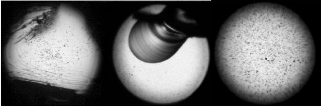
Figure 1 Types of damage to endoscope lenses: Lens break, sliver, water vapor. (Courtesy Storz Germany)<sup>1</sup>.
