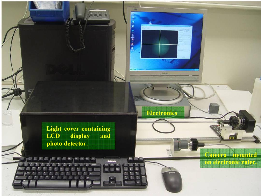
Figure 3 Overview of endoscope test bench.
