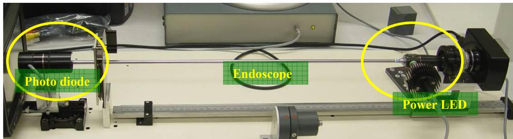
Figure 2 Measurement transmission illumination fibers.
