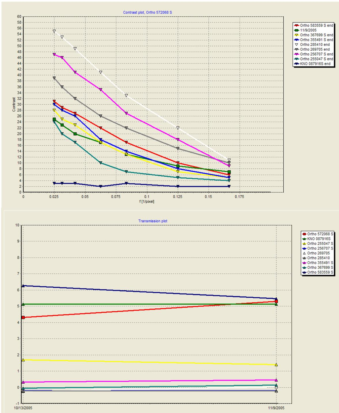
Figure 5 Contrast plots of eight different endoscopes of type Storz 28721 BWA at several stages of usage. The transmission of the illumination fibers of endoscopes with numbers 285410, 355491, and 367699 are so low, that they should be removed from clinical use.
