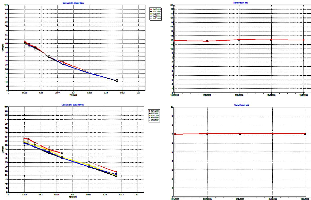
Figure 4 Reproducibility of contrast plots (left) and illumination fiber transmission (right) of five endoscope measurements by repeatable repositioning endoscope, target LCD display angle and camera. Upper row: endoscope with 0° view angle, bottom row: endoscope with 90° view angle.
