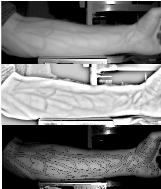
Figure 6 Effect of digital enhancement on an infrared picture of the forearm: Top, original infrared image. Middle: Enhanced image by changing contrast settings in Microsoft Word. Bottom: Results of vein segmentation using Laplace operator (Threshold value=0).
