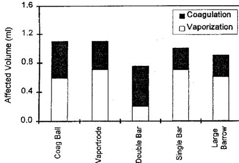
Figure 2. Tissue effects after application of five different EVAP-elements at 300 Watt.
