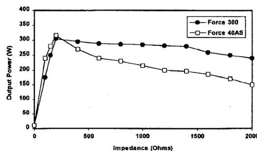
Figure 1. Influence of the impedance between active and return electrode on the output power at a fixed power setting of 300 Watt (monopolar, pure cut mode) for the Force 40 and the Force 300 electro surgical generators (both Valleylab)<sup>1,2</sup>.
