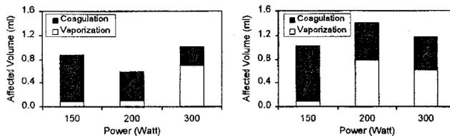
Figure 4 Tissue effects after application of the Prosurg single Rollerbar at 1 mm/s with the Force 40 (left) and the Force 300 (right) at different powers.
