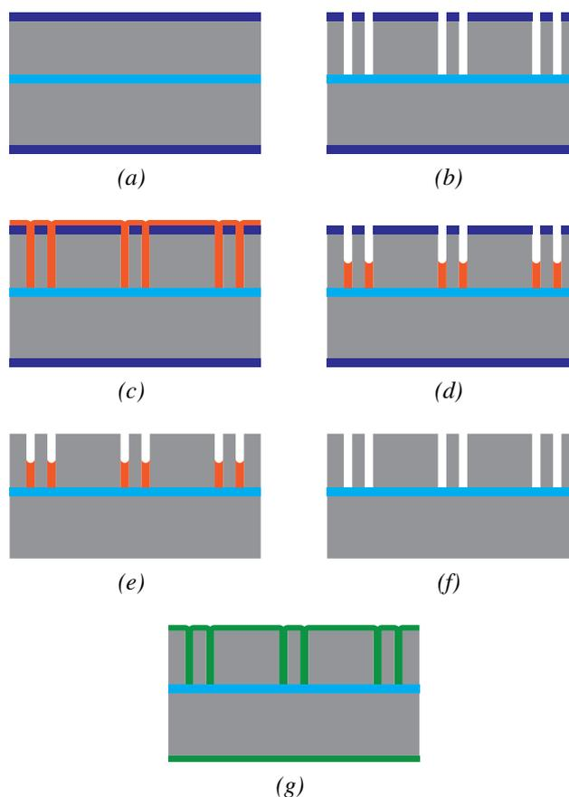
Figure 3: Schematics of the etch stop and channel outline formation in the TASCT process, with the steps (a) thermal oxidation of a SOI wafer, (b) RIE of  $\text{SiO}_2$  and notching-free DRIE of Si, (c) CVD of parylene-C, (d) etching of parylene-C in an  $\text{O}_2$  plasma, (e) stripping of the  $\text{SiO}_2$  hard mask in buffered HF, (f) stripping of the remaining parylene-C in piranha, (g) trench refill with LPCVD of low-stress SiRN.
