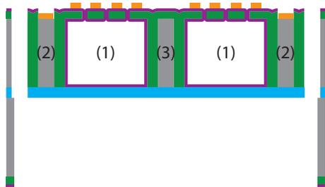
Figure 7: Channel release etch via a combined directional process (Bosch) and isotropic process (SF<sub>6</sub> plasma). In the image, (1) is indicating the channel, (2) is indicating the Si side wall heating structures, and (3) indicates an in-channel pillar.
