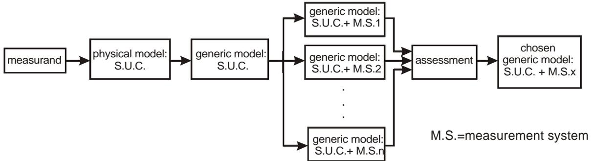
**Figure 2.** Sketch of the knowledge based system at top-level
