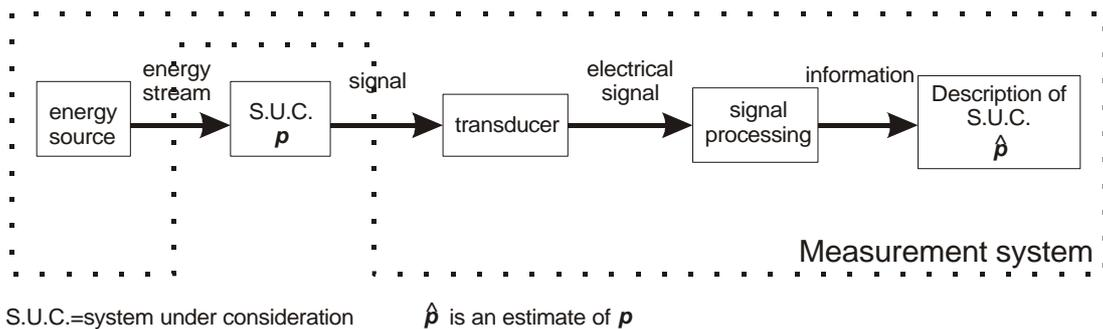
Figure 1. Sketch of a standard measurement system
