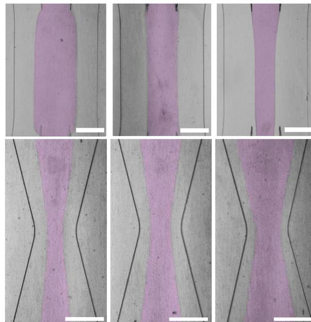
**Figure 3:** Patterned devices with collagen gel (artificially colored pink). Gel is cured and fluidic access channels are filled with 1xPBS solution. (top) straight devices (bottom) tapered devices. Different flow ratios during patterning result in the different gel widths. Flow ratios are 1:2:1 (left) 1:1:1 (middle) and 1:0.5:1
