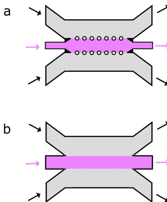
**Figure 1:** Schematic top view representations of angiogenesis-on-chip devices. The gray areas are microfluidic channels, arrows indicate fluidic inlets and outlets and purple regions indicate collagen-filled volumes. (a) Conventional devices contain micropillars for patterning gels[1]. (b) The same gel geometry can be created by surface coating during hydrodynamic focusing.
