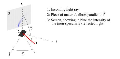
Figure 5. Example of reflective behaviour described by BRDF
