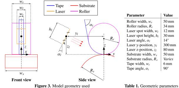
Light hitting the roller is assumed to reflect specularly, with the reflectivity being a function of the angle of incidence according to the Fresnel equations. A roller with a polytetrafluoroethylene (PTFE) coating
