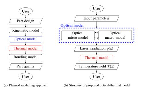
Figure 2. Overview of LATW process model
