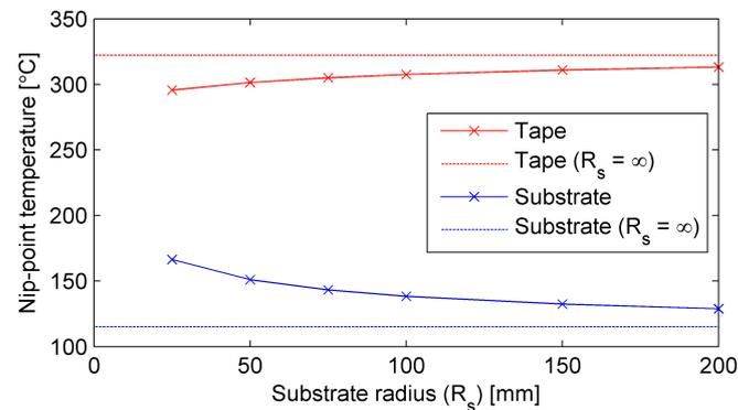
**Figure 7.** Nip-point temperatures as a function of substrate curvature
