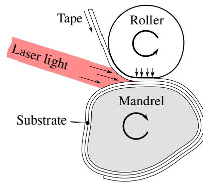
**Figure 1.** Schematic overview of the LATW process.
