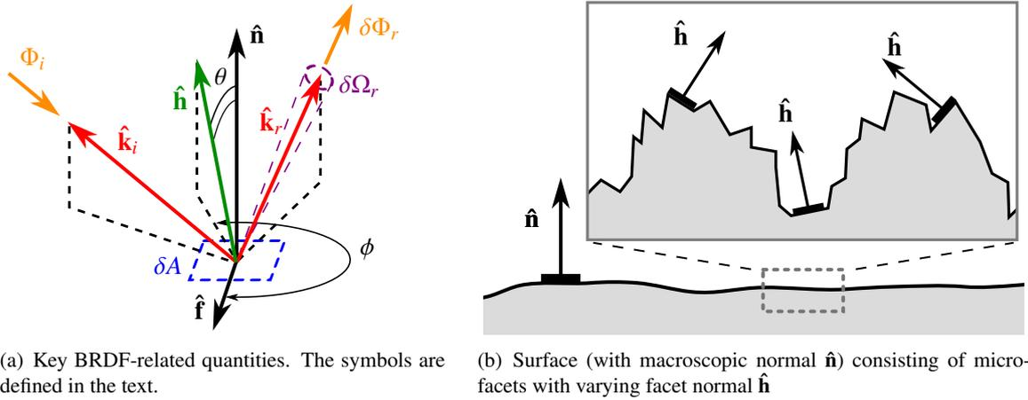
**Figure 4.** Illustration of the principles behind the BRDF
