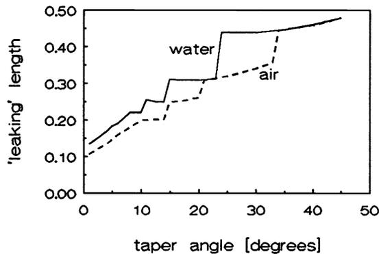
**Figure 4:** 'Leaking' length along the scalpel where rays refract out of the scalpel in relation to the taper angle in air (dotted curve) and water (solid curve). The 'leaking' length was normalized with respect to the total length of the scalpel relative to the tip.
