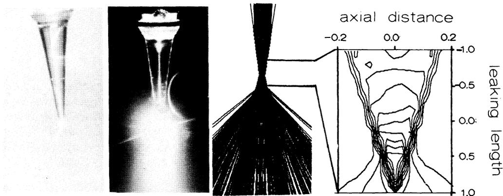
*Figure 2: From left to right panel: photo scalpel, calculated beam, photographed beam and irradiance distribution of the 16 degree tapered scalpel (MTRP 5.0, Surgical Laser Technologies, Malvern, PA, USA) in water.*
