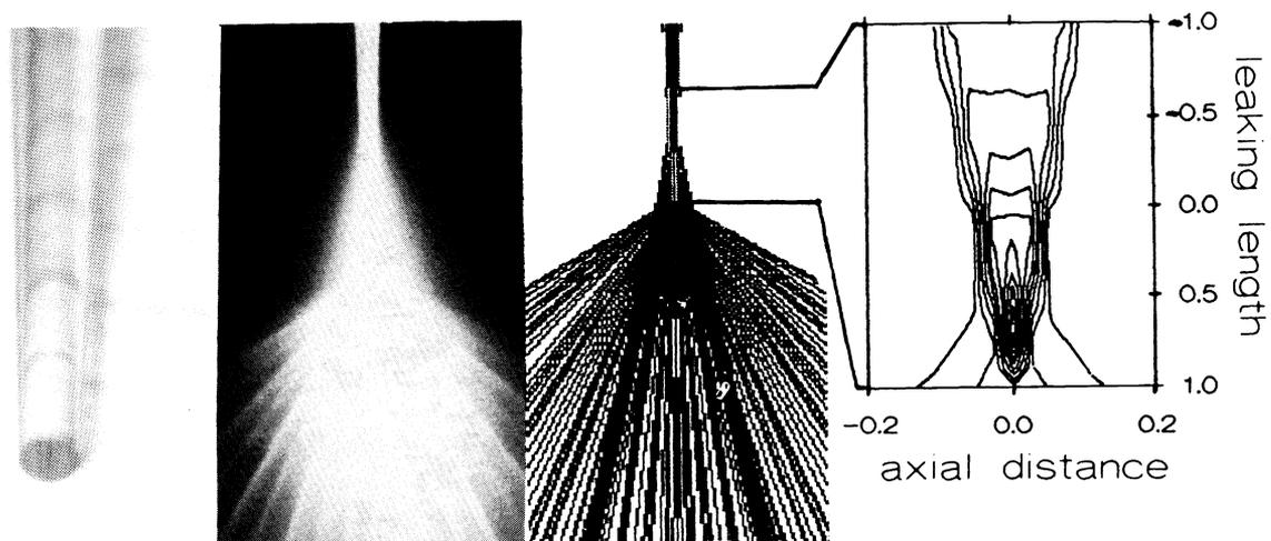
*Figure 3: From left to right panel: photo scalpel, calculated beam, photographed beam and irradiance distribution of the 4 degree tapered scalpel with a flat tip in water.*
