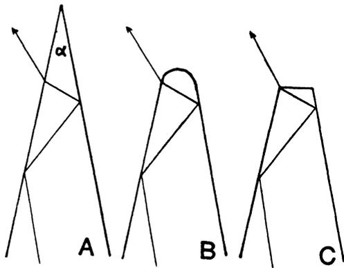
*Figure 1: (A) A ray will be reflected up and down inside a tapered rod with angle  $\alpha$  until the angle of incidence relative to the surface exceeds the critical angle and the ray is refracted out of the scalpel. The point of the tapered rod may end in either a hemispherical (B) or a flat tip (C).*
