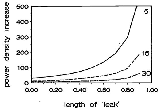
**Figure 5:** increase in power density relative to the power density at the entrance of the scalpel for 5, 15, and 30 degrees taper angles. The 'leaking' length was normalized with respect to the total length of the scalpel relative to the tip.
