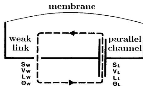
Figure 1. Two-hole resonator. The flexible membrane has area  $S$  and deflection  $d$ . The dashed line marks the superfluid loop threading the two holes.
