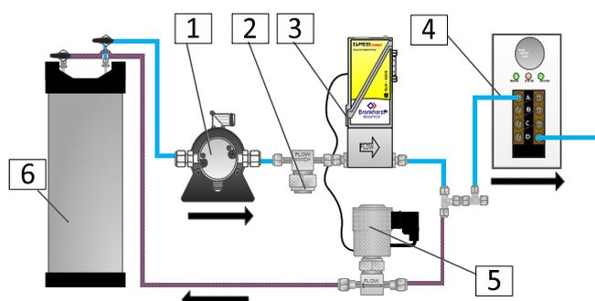
Figure 2. Schematic of pump driven flow generation with pump(1), filter(2), pressure sensor(3), degasser(4), bypass control valve(5) and liquid storage tank(6).
