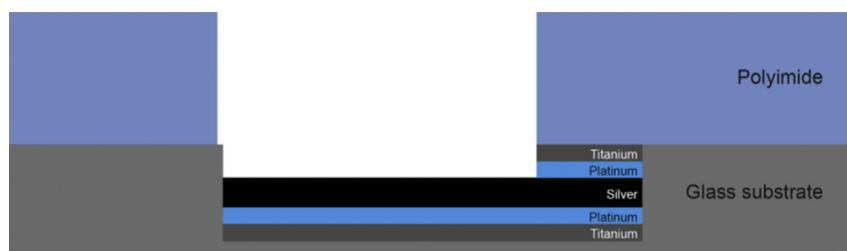
Fig. 4. Cross-section of the structure of the chip design. Shown thicknesses are not drawn to scale.
