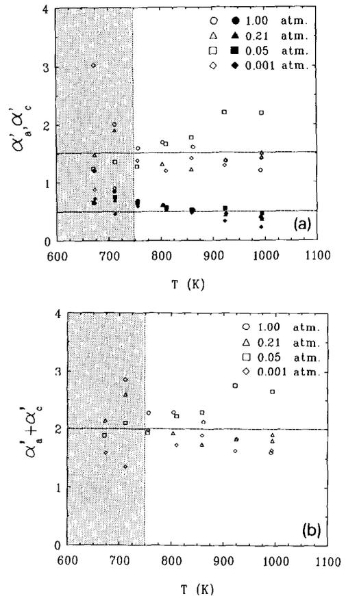
Fig. 4. (a) Anodic (open symbols) and cathodic (closed symbols) charge transfer coefficients for the gold gauze electrodes as a function of temperature and  $P_{O_2}$ . (b) Sum of the charge transfer coefficients. The shaded areas indicate the temperature region where hysteresis in the polarization behaviour occurs (see also ref. [1]).
