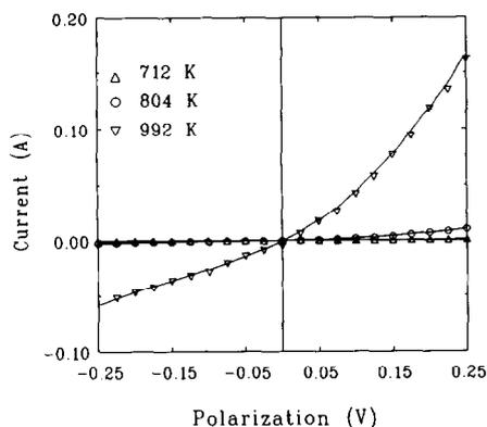
Fig. 1. Typical examples of current–voltage curves for BE25 with co-pressed gold gauze electrodes measured in air.
