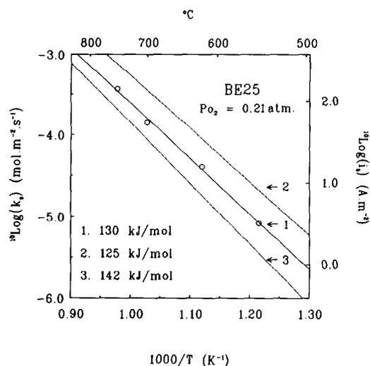
Fig. 7. Comparison of the surface oxygen exchange rate  $k_s$  (1, left vertical axis), established from isotope exchange experiments [10], with the exchange current densities (right vertical axis) for BE25/gold gauze (2) and BE25/gold sputtered electrodes (3).
