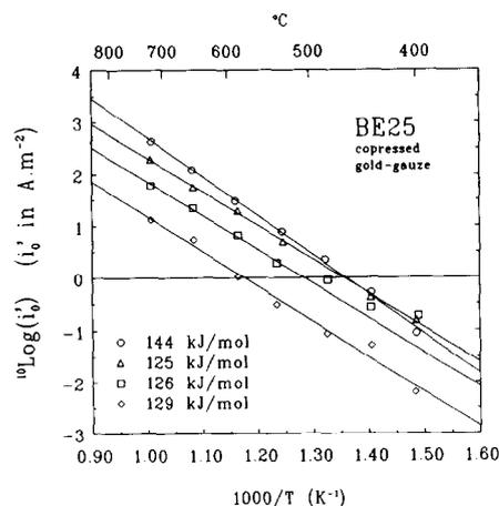
Fig. 2. Oxygen exchange current densities for BE25 with gold gauze electrodes measured at different oxygen partial pressures:  $P_{\text{O}_2} = 1.0$  atm ( $\circ$ ), 0.21 atm ( $\Delta$ ), 0.05 atm ( $\square$ ) and 0.001 atm ( $\diamond$ ).
