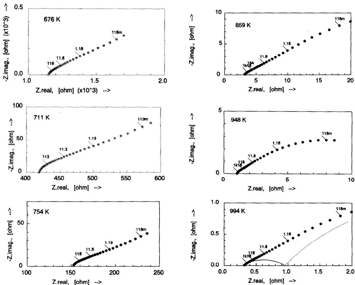
Fig. 5. Impedance diagrams for the BE25/gold gauze electrode measured in air as a function of temperature: (( $\star$ ) measured data points, ( $\circ$ ) results from NLLSF analysis). Frequencies are in Hz. For the measurement at 994 K the drawn line represents the contributions to the dispersion of the separate sub-circuits.
