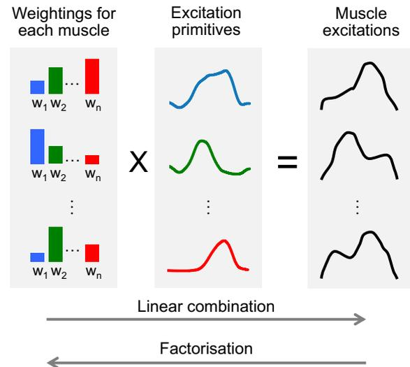
**Fig. 2.** Excitation primitives and weighting factors from factorisation of experimental excitations can be used as input for CEINMS. CEINMS neural mapping is integrated in the software and can be configured to linearly combine excitation primitives and weightings.
