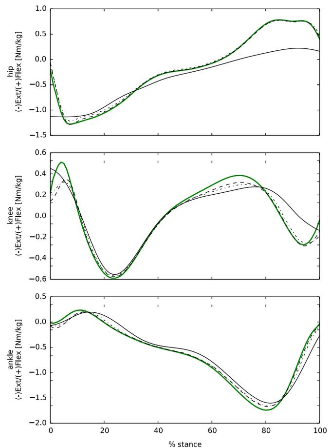
**Fig. 7.** Comparisons between experimental joint moments from OpenSim inverse dynamics (solid green) and joint moments predicted by EMG-driven (solid black), EMG-assisted (dash-point), and static optimisation (dashed) modes for hip, knee and ankle flexion extension during stance phase. (For interpretation of the references to color in this figure legend, the reader is referred to the web version of this article.)
