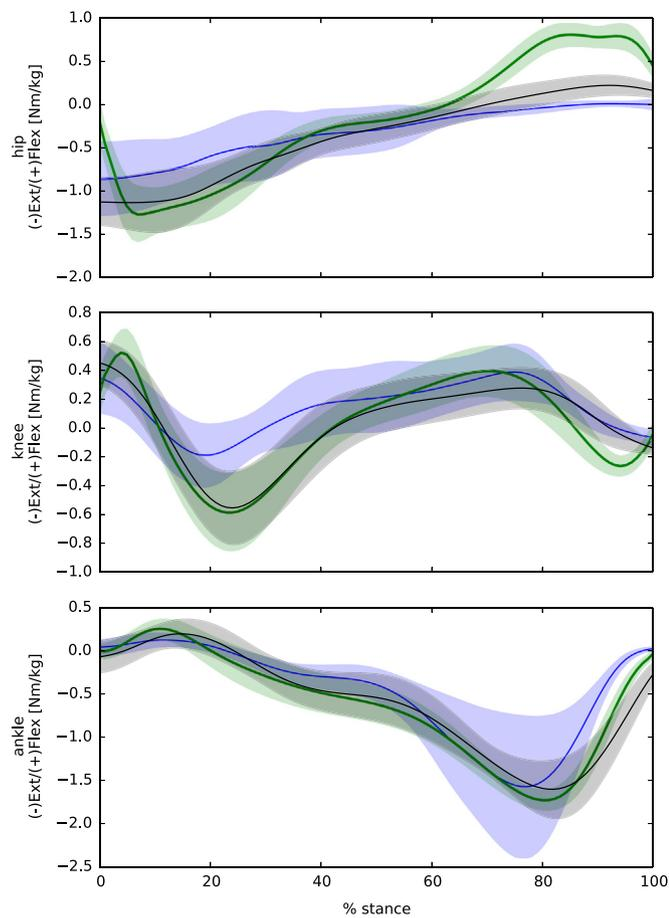
**Fig. 6.** External joint moments from OpenSim inverse dynamics (green), calibrated EMG-driven (black), and uncalibrated EMG-driven (blue). The curves represent the ensemble average (shaded area 1STD) of 30 walking trials from 5 different individuals. These results were from trials different to those used to calibrate CEINMS. (For interpretation of the references to color in this figure legend, the reader is referred to the web version of this article.)
