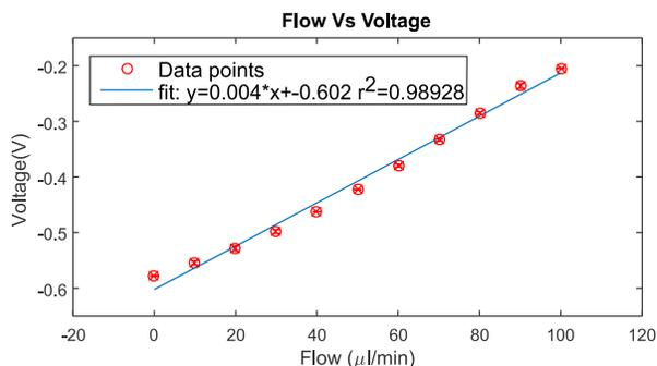
Figure 4: Flow characterization ( $R^2=0.98928$ ), Error bars indicate the hysteresis over the 1 repetition of the reference flow pattern.
