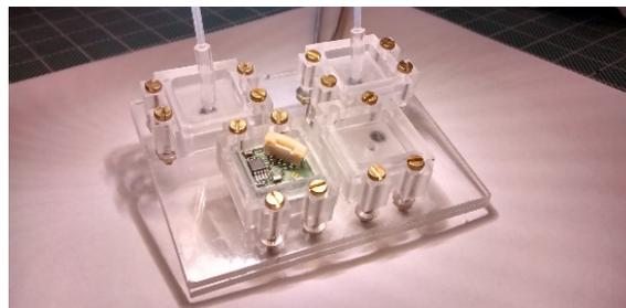
Figure 3: Fluidic circuit board (FCB) with mounted MFBBs, developed for testing purposes as shown in fig4.
