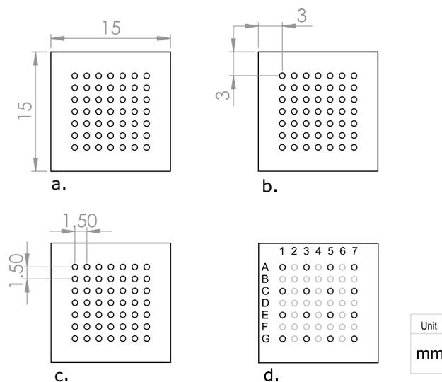
Figure 1: Standardized dimensions as proposed in ISO workshop document [6]: a. MFBB outline dimensions, b. Grid starting position, c. Grid pitch and d. Port annotation and preferred (bold) port positions.
