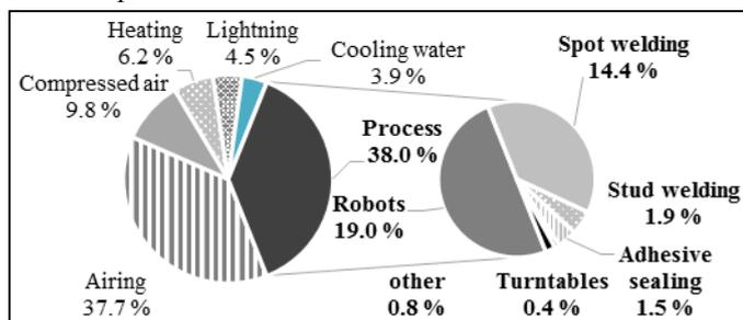
Fig. 5. Electrical energy consumption share in body shop
