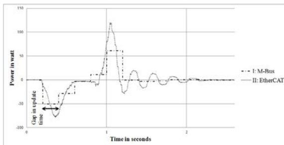
Fig. 8. Load profiles of an industrial robot recorded by EtherCAT with a data rate of 50 Hz and M-Bus with a maximal data rate of 5 Hz
