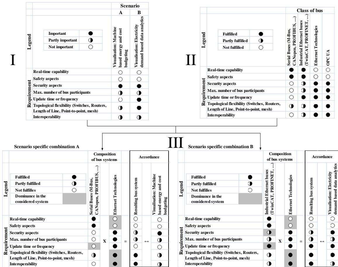
Fig. 5. Evaluation matrices for bus systems and desired functions over correspondent requirements and the combination of both
