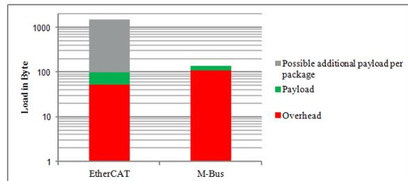
Fig. 6. Ratio of payload to overhead for transmission of actual power, voltage, current and phase shift over an EtherCAT and an M-Bus line from A/D converter to signal converter (S/C)
