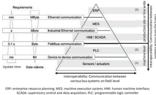
Fig. 2. Communication structure within a factory with requirements regarding data update time and data volume
