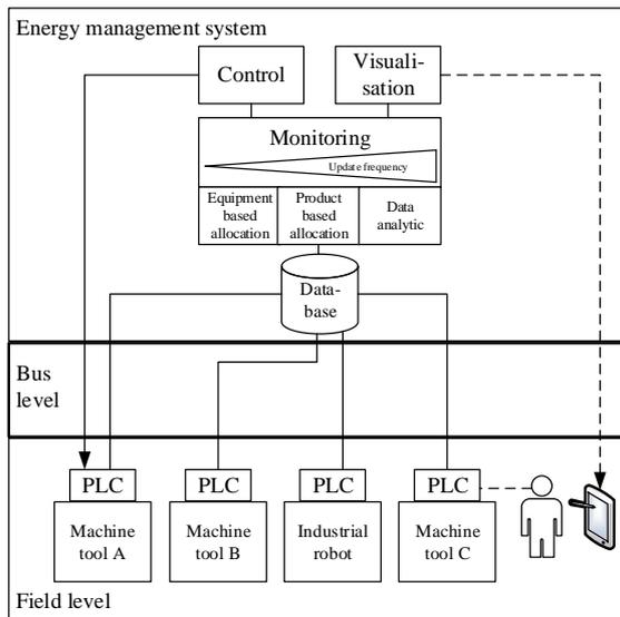
Fig. 1. Possible structure of an energy management system
