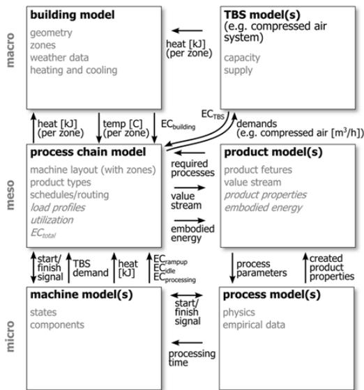
Fig. 5. Framework for multi-level modeling and simulation
