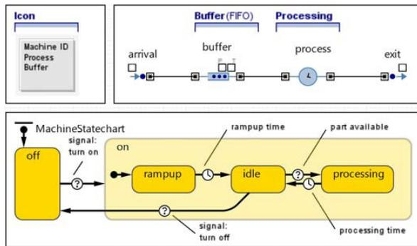
Fig. 8. Machine object model: Top: Enterprise library elements for buffering and processing of product entities; Bottom: Operational states of the machine.
