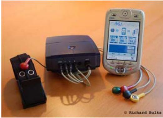
Figure 11 shows a COPD BAN, where the MBU is implemented by a PDA (a Qtek). This BAN is equipped with a respiration sensor and 3-channel ECG. These are examples of front end supported sensors systems. The box in the centre is the sensor front end. This configuration represents one of many different specialisations of the generic BAN developed and realised at the University of Twente.
