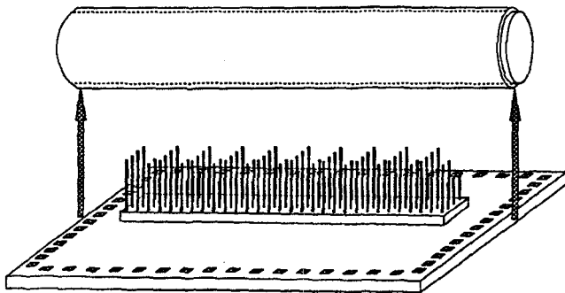
Figure 1: Schematic overview of a CMOS chip carrying a three-dimensional array of 128 microelectrodes, which can be inserted into a nerve
