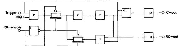
Fig. 1. Circuit diagram of the ring oscillator/inverter chain.
