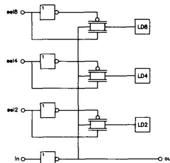
Fig. 2. Circuit diagram of a delay element  $\tau$ .
