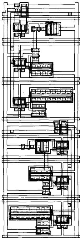
Fig. 4. Chip lay-out of a delay element.
