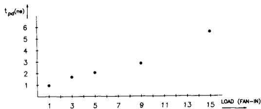
Fig. 3. Propagation-delay versus load for the inverter chain.
