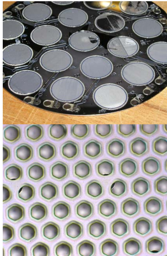
Fig. 2. Top: picture of the InGrid wafer. There are 19 fields each with a different grid geometry. Note the individual anode and grid connections at the edge of the wafer. Bottom: The InGrid pattern which was used for the measurements. Note the slightly hexagonal holes (hole pitch 60 \mu\text{m} ). The insulating pillars (diameter 30 \mu\text{m} ) are centred between three adjacent holes, and are just visible. No local loss of sensitivity is expected.
