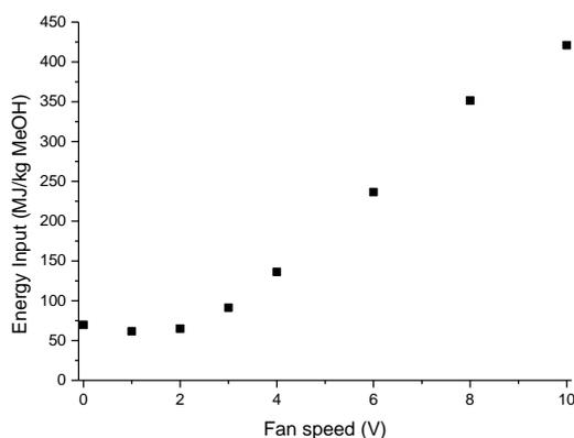
**Figure 10** Energy input per kg of methanol as a function of fan speed. (P=50 barg, Catalyst bed outlet=468K, Condenser outlet temperature=363K, Feed gas 2)
