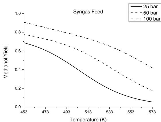
**Figure 1** Chemical equilibria in methanol synthesis from syngas feed. Syngas feed:  $H_2/CO/CO_2$  75.9/16.9/7.2
