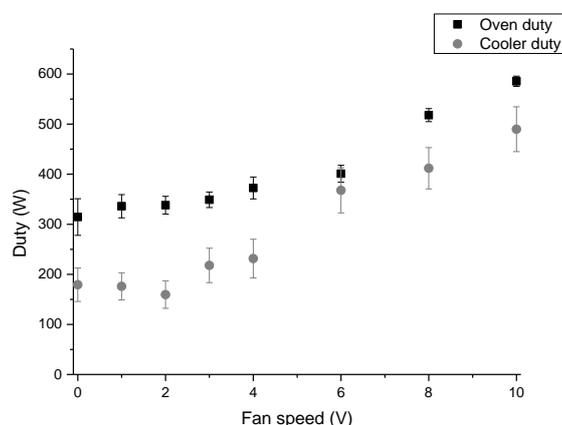
**Figure 9** Oven and cooler duty as a function of fan speed. (P=50 barg, Catalyst bed outlet temperature=468K, Condenser outlet temperature=363K, Feed gas 2)
