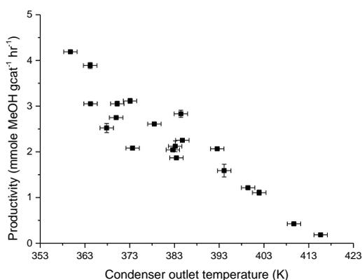
**Figure 6 Reactor productivity as a function of condenser outlet temperature. (P=50 bar, Catalyst bed outlet temperature =483K, Catalyst bed pressure drop=0.15mbar, Feed gas 1)**
