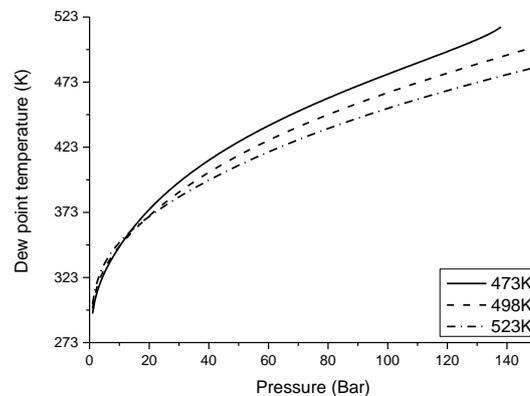
Figure 3 Dew point of the equilibrium mixture at 473/498/523K as a function of pressure. (CO<sub>2</sub> feed: H<sub>2</sub>:CO<sub>2</sub> 3:1)
