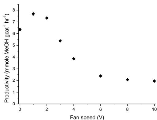
**Figure 7 Reactor productivity as a function of fan speed. (P=50 barg, Catalyst bed outlet temperature=268K, Condenser outlet temperature =363K, Feed gas 2)**
