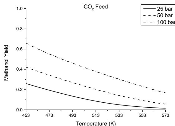
**Figure 2** Chemical equilibria in methanol synthesis from  $CO_2$  feed.  $CO_2$  feed:  $H_2/CO/CO_2$  75.0/0/25.0
