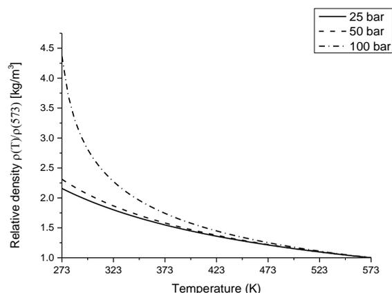
**Figure 4** Relative density  $\rho(T)/\rho(573)$ , calculated for the equilibrium composition generated at 503K and resp. 25/50/100 bar ( $\text{CO}_2$  feed:  $\text{H}_2:\text{CO}_2$  3:1).
