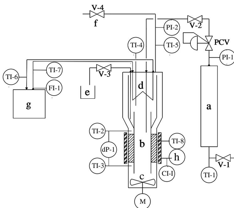
**Figure 5 Schematic overview of the setup: (a) Buffer vessel, (b) Catalyst Section (annulus), (c) Fan, (d) Cooler, (e) Liquid Outlet, (f) Purge, (g) water bath, (h) oven temperature controller, (TI) Temperature Indicator, (PI) Pressure Indicator, (CI) Current Indicator, (dP) differential Pressure Indicator, (FI) Flow Indicator, (PCV) Pressure Control Valve, (V) Valve.**
