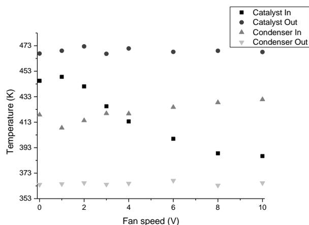
**Figure 8 Gas temperatures at the catalyst and condenser inlet/outlet as a function of fan speed. (P=50 barg, Catalyst bed outlet temperature=468K, Condenser outlet temperature =363K, Feed gas 2)**
