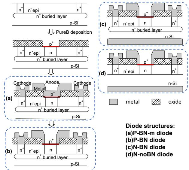
**Fig. 1.** Schematics of the 4 different diode structures under investigation. Left: The basic process flow for the fabrication of PureB SPADs with n<sup>+</sup> plugs to a buried n<sup>+</sup>-layer on a p-type Si substrate, with the diode before (a) and after (b) metal removal. Right: Diodes fabricated on an n-type Si substrate with (c) and without (d) a buried n<sup>+</sup> layer.[5]
