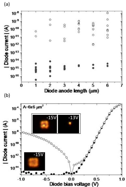
**Fig. 11.** (a) The current measured at 1 V reverse bias for sets of 12 diodes (6 P-BN and 6 P-BN-m) as a function of diode length, grouped in closed circles for ideally low currents and open circles for high reverse currents. (b)  $I$ - $V$  characteristics of two P-BN devices and images of their AM light emission patterns.
