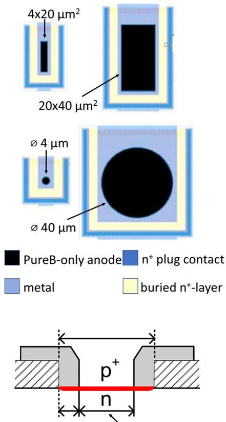
**Fig. 2.** Top: Examples of the PureB diode layouts for rectangular and circular light-entrance windows. Below: A schematic cross section of the metal contacting scheme of PureB diodes with an n-enrichment implantation. The  $L$  and  $W$  indicate the length and width, respectively, of the light entrance windows. For all the available anodes sizes, a  $\Delta L = \Delta W = 0.5 \mu\text{m}$ ,  $1.0 \mu\text{m}$  and  $1.5 \mu\text{m}$  was implemented.
