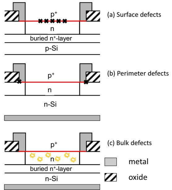
**Fig. 7.** Illustration of the three types of defects identified in the investigated PureB diodes. (a) Surface pitting seen on some diodes before treatment with wet-etch steps, and enhanced by TMAH etching, (b) perimeter pits seen on all diodes but only after TMAH etching, (c) bulk defects that were related to extra surface roughness but identified as bulk defects only through optoelectrical measurements.
