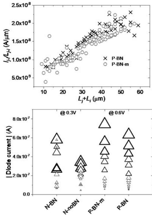
**Fig. 9.** (a) The differential forward current at 0.3 V for all the 16 sizes of square P-BN and P-BN-m devices as a function of the sum of light-entrance window lengths  $L_j+L_i$ . (b) The forward diode current measured on 16 square diodes with  $L = 1 \mu\text{m}$  to  $40 \mu\text{m}$ , at 0.3 V for N-BN and N-noBN diodes, and at 0.6 V for P-BN and P-BN-m diodes. The symbol sizes are directly proportional to  $L$ .
