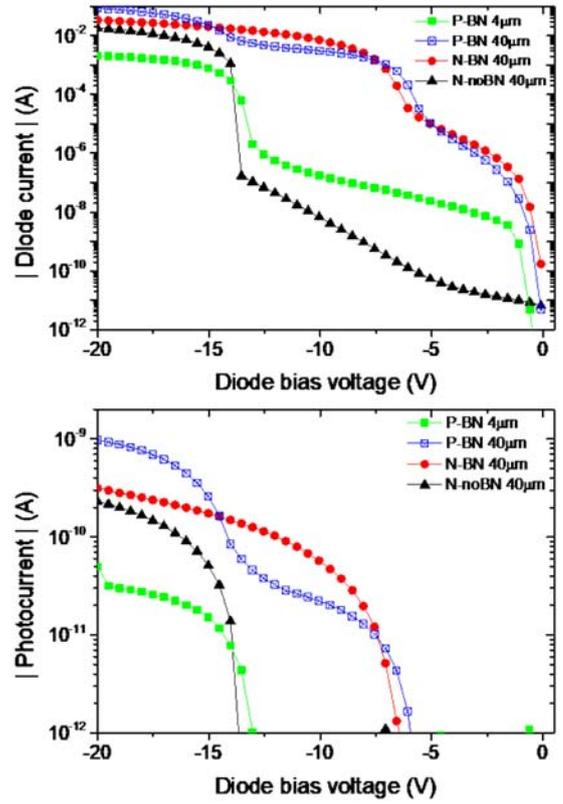
Fig. 5. Typical reverse  $I$ - $V$  characteristics for P-BN, N-BN, and N-noBN diodes (top), and the photocurrents simultaneously measured using Setup A (bottom).
