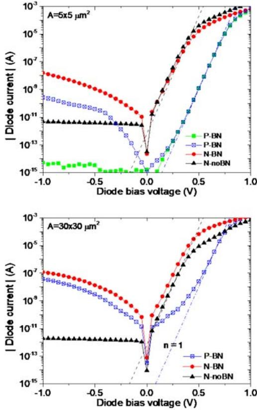
Fig. 4. Typical  $I$ - $V$  characteristics measured on P-BN, N-noBN and N-BN diodes with sizes  $5 \times 5 \mu\text{m}^2$  (top) and  $30 \times 30 \mu\text{m}^2$  (bottom). Dashed lines indicate the ideality factor  $n = 1$  relationship.
