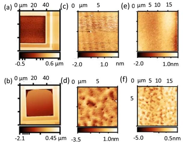
**Fig. 10.** AFM scans of n-type diode surfaces before and after etch tests. An N-BN diode before (a) and after (b) TMAH etching upon which etch pits appear in the corners. Anode surface scans for an N-noBN (c) and an N-BN (d) diode after TMAH-etching, and an N-noBN (e) and an N-BN (f) diode after PureB removal.
