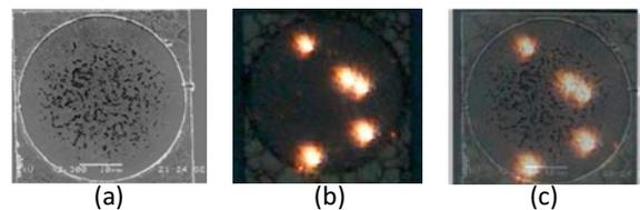
**Fig. 8.** Images of a circular P-BN diode with diameter 40  $\mu\text{m}$ , taken with (a) the SEM, and (b) setup B during a reverse biasing of 15 V. In (c) an overlay is shown of (a) and (b).
