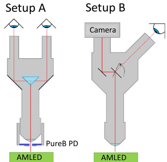
**Fig. 3.** Schematics of the 2 setups used for on-wafer biasing and monitoring of light emission from the diodes-under-test. Setup A: a PureB photodiode was mounted on the objective of the probe-station microscope to measure AM light emission; setup B: a camera is mounted on the microscope ocular for imaging of light emission across the diode surface.
