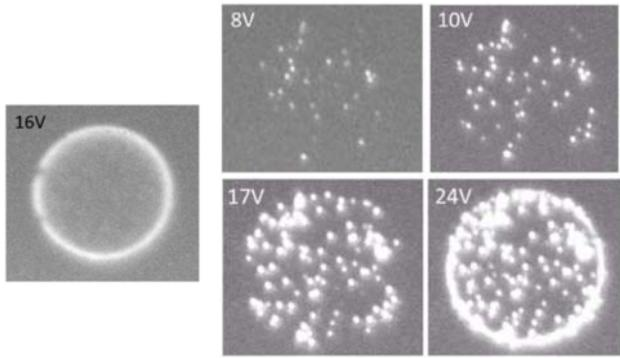
**Fig. 6.** Camera images of the light emission from reverse-biased circular N-noBN (left) and N-BN (right) diodes with a diameter of 40  $\mu\text{m}$ . The applied bias voltage is given in each image.
