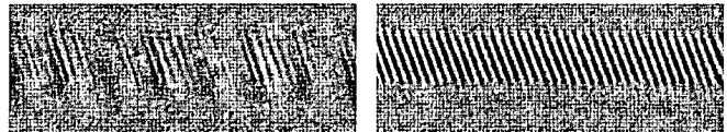
Fig. 3. MFM images ( 7.5 \mu\text{m} \times 20 \mu\text{m} ) corresponding to the overwrite sequences with ME tape from Fig. 2 (left image: I_{ovr} = 10 \text{ mA}_{pp} ; right image: I_{ovr} = 30 \text{ mA}_{pp} ).
